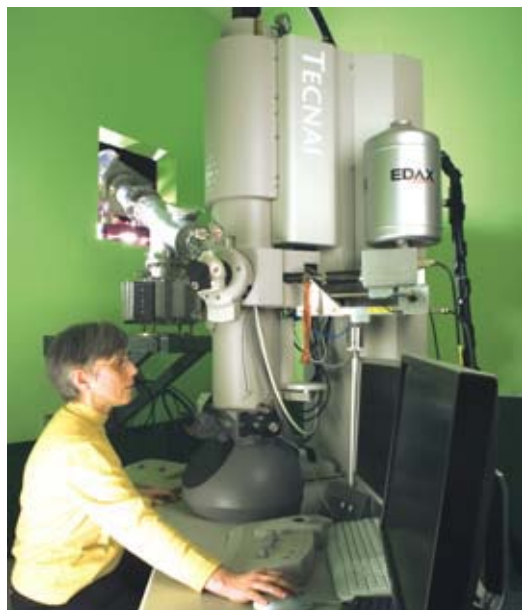
CSNSM's new transmission electron microscope will make it possible to observe the microstructural evolution of a sample during its simultaneous irradiation by two ion beams. The microscope column will receive two lines of energetic ion beams, directed symmetrically with respect to each other. The line from the ARAMIS accelerator may be seen. Construction of the line from the IRMA implanter is under way.
